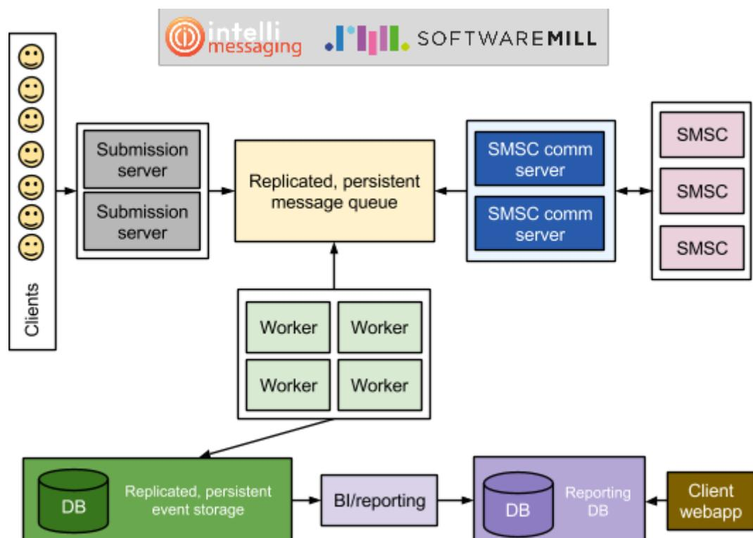
Each component is independent, can be scaled independently, and doesn't have to work at the same time as the other components. This is especially important for the SMSC communication servers, which connect to third-party providers; such links are inherently unreliable, and can go up and down unpredictably.
